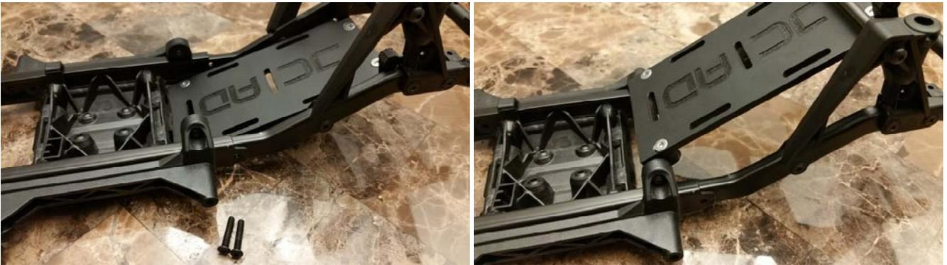
4. Mount the SWB Front Mount to the stock shock towers using the 10mm flat head screws.
