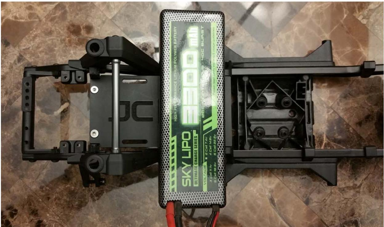
*Tech Tip: place a couple pieces of Velcro between the battery and the plate to prevent the battery from moving around.*
