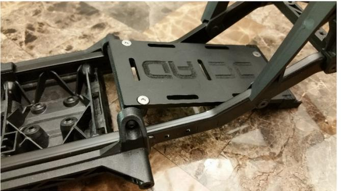
4. Mount the Front Mount to the stock rear servo mount using the 10mm flat head screws.
