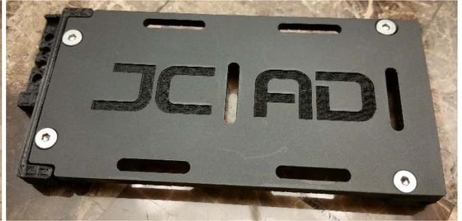
3. Mount the Rear Mount to the stock battery box mount using the screws and bushings from step 1.
