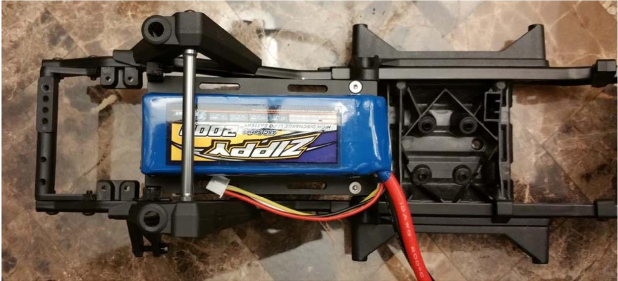
**Transverse:** Max battery size (L x W x H): 140mm+ (5.5"+) x 60mm (2 3/8") x 50mm+ (2"+)
